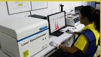
Spectrometric analysis in progress (Ultimheat Laboratory)
