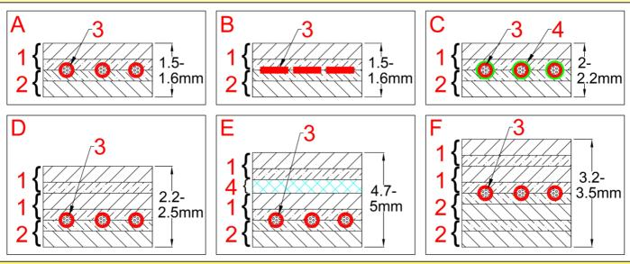
1: Fiberglass reinforced silicone compound of the upper face; 2: Fiberglass reinforced silicone compound of the lower face; 3: Heating wires; 4: Metal mesh wire for grounding and mechanical reinforcement; 5: FEP Primary insulation of heating wires.
