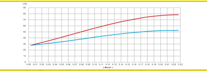
Variation, as a function of the power in W/cm<sup>2</sup> of the silicone heating ribbon, of the wall temperature of an empty, non-thermally insulated PVC tube
