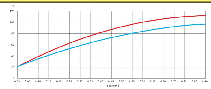
Variation, as a function of the power in W/cm<sup>2</sup> of the silicone heating ribbon, of the wall temperature of a stainless-steel tube, filled with non-circulated water, no-thermally insulated
