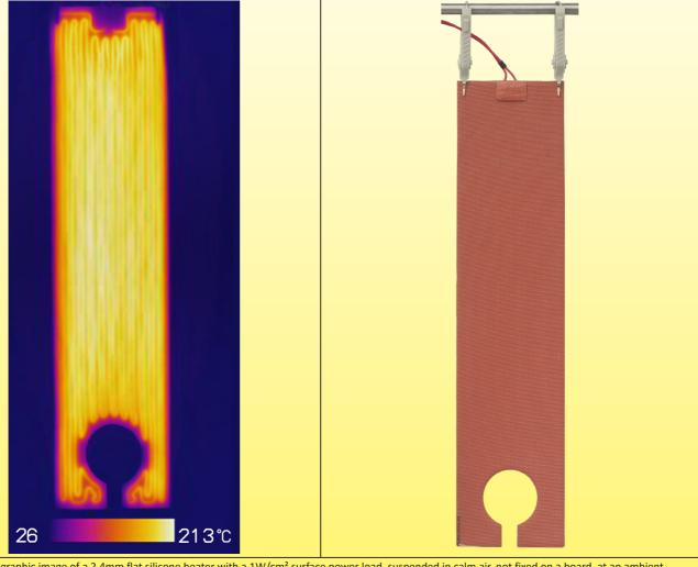
Thermographic image of a 2.4mm flat silicone heater with a 1W/cm² surface power load, suspended in calm air, not fixed on a board, at an ambient temperature of 25°C. The surface temperature reaches 213°C, nearby its destruction.
