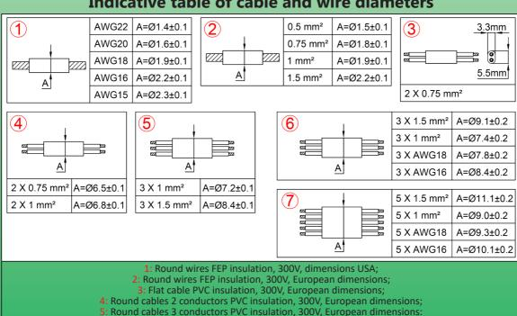
6: Round cables 3 conductors rubber insulation 300V, European and USA dimensions. 7: Round cables 5 conductors rubber insulation 300V, European and USA dimensions.
