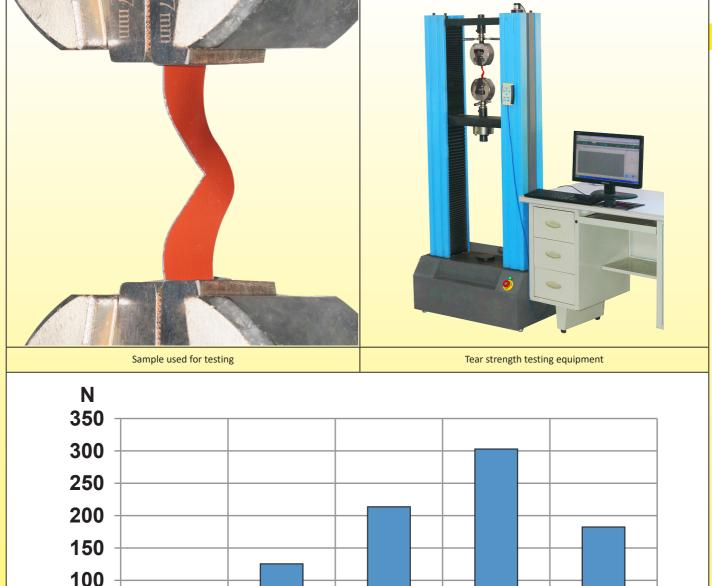
Comparative tear strength of the different thicknesses models 1: 0.8mm; 2: 1.6mm; 3: 2.3mm; 4: 3.2mm; 5: 2.3mm with stainless steel mesh reinforcement
