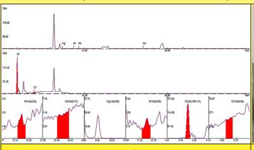
Rohs spectrogram of a fiberglass reinforced silicone sheet (Ultimheat laboratory)
