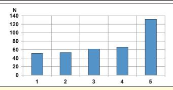
Comparative elongation strength at 0.05mm/min of the different thicknesses models 1: 0.8mm, 2: 1.6mm, 3: 2.4mm, 4: 3.2mm, 5: 2.4mm with stainless steel mesh reinforcement
