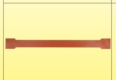
Type of sample tested (350 × 35mm)
